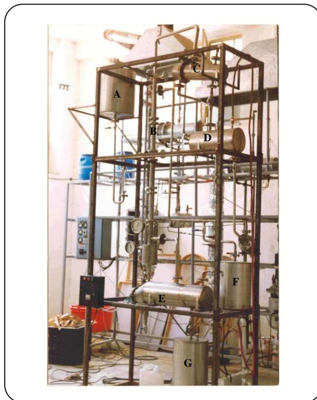
*Fig. 1: Picture of the distillation pilot plant A. feed vessel B. distillation column C. condenser D. decanter E. reboiler F. vessel for product from top of column G. vessel for product from bottom of column.*
