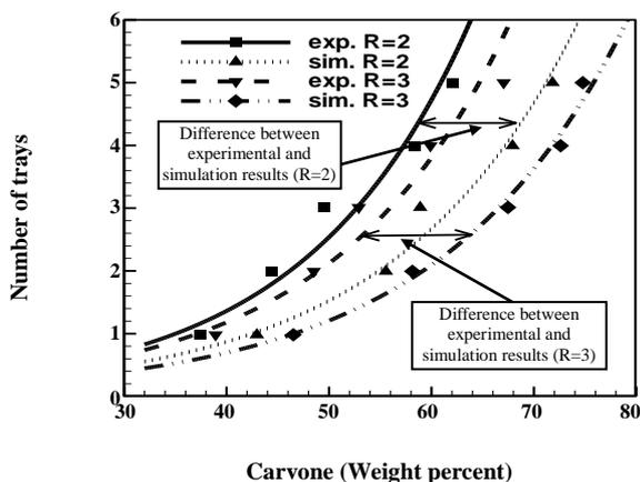
Fig. 3: A comparison between experimental and numerical results (PSRK eq.) for the evolution of carvone separation (separation percent vs. number of trays) A. experimental results (R=2) B. numerical results (R=2). C. experimental results (R=3) D. numerical results (R=3).
