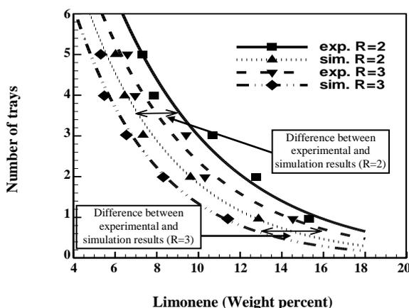
Fig. 5: A comparison between experimental and numerical results (PSRK eq.) for the evolution of limonene separation (separation percent vs. number of trays) A. experimental results (R=2) B. numerical results (R=2). C. experimental results (R=3) D. numerical results (R=3).
