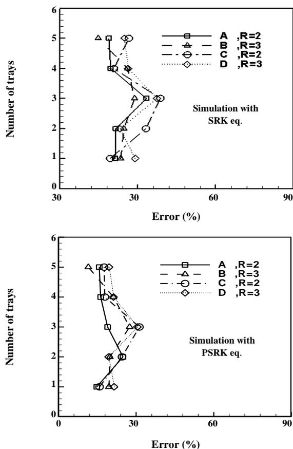
Fig. 6: The percent error between the results of computer simulations (SRK and PSRK eqs.) with experimental results. A. Carvone enrichment with  $R=2$  B. Carvone enrichment with  $R=3$ . C. Limonene removal with  $R=2$  D. Limonene removal with  $R=3$ .
