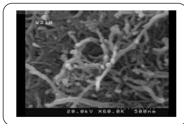
Fig. 2: FESEM results of MWCNT-Fe 3 O 4 nanocomposite.
