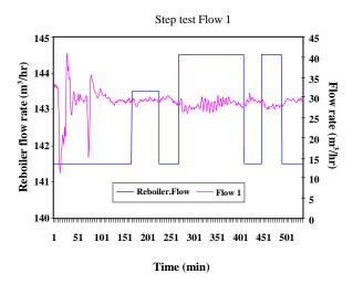
Fig. 8: Flow 1 Light Naphtha flow to storage.
