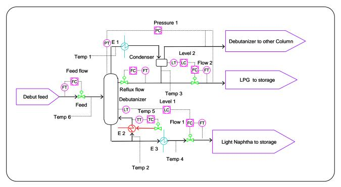
Fig. 2: Debutanizer column configuration.
