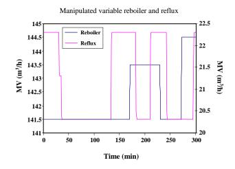
Fig. 22: Manipulated variable reboiler and reflux flow rate.
