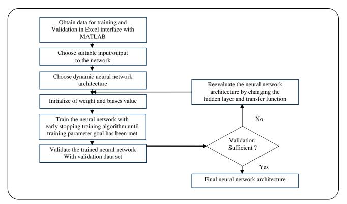
Fig. 5: Procedure of the neural network architecture.
