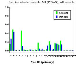
Fig. 18: Component contribution plot reboiler flow rate.
