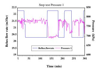
Fig. 13: Pressure 1 Debutanizer receiver overhead pressure.
