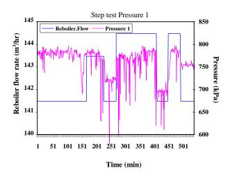
Fig. 9: Pressure 1 Debutanizer receiver overhead pressure.
