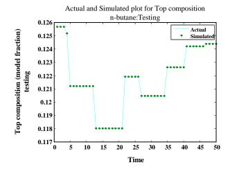
Fig. 23: Actual and simulated n-butane at the top composition for testing.
