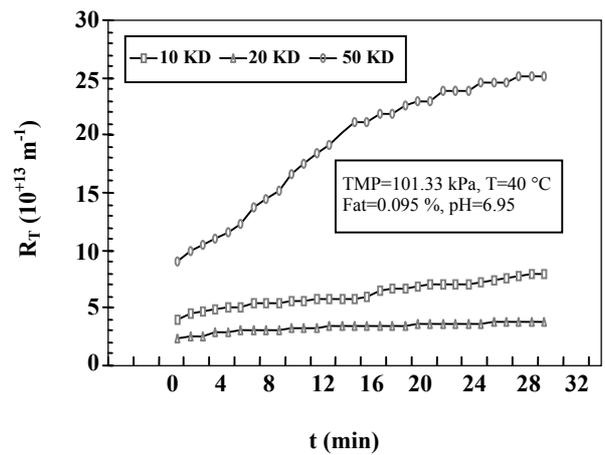
Fig. 5: Dynamic behavior of total hydraulic resistance ( $R_T$ ) as a function of MWCO during ultrafiltration of skim milk.
