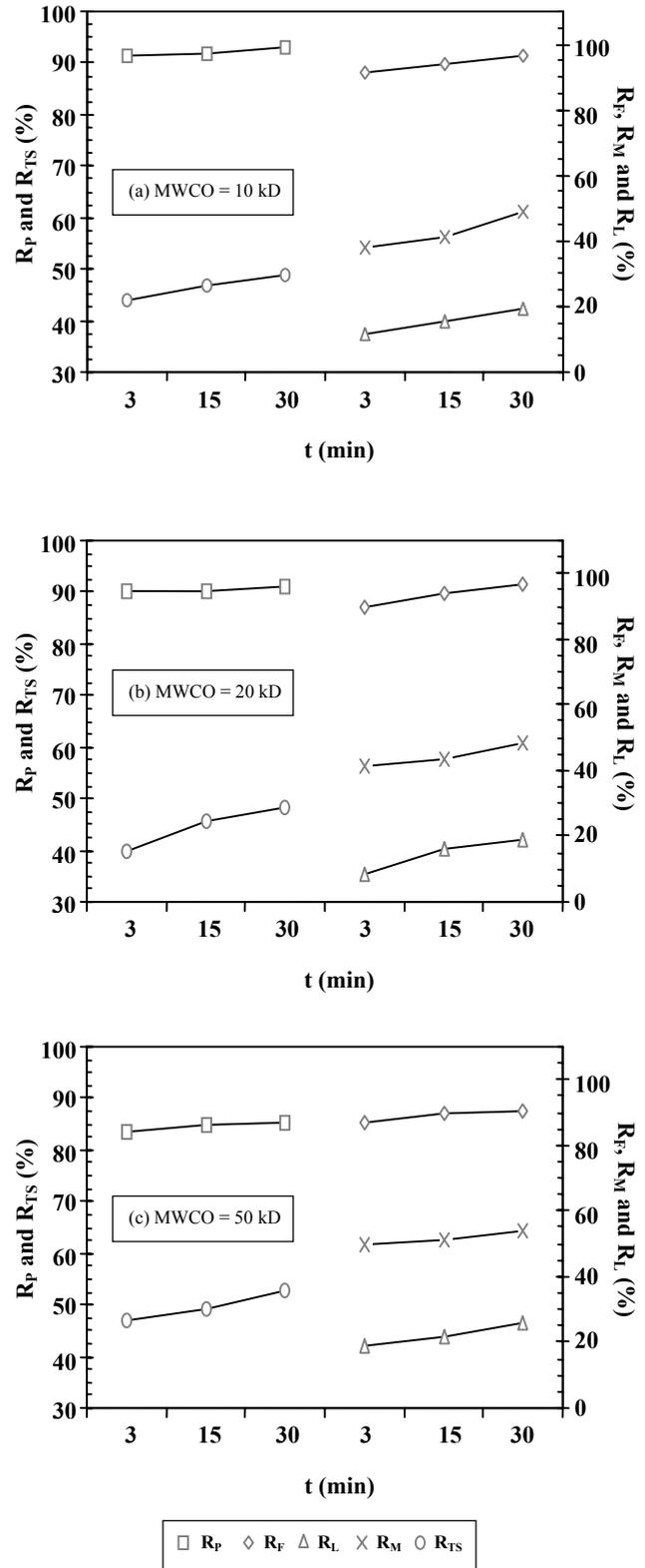
Fig. 7: Dynamic behavior of solutes rejection (protein,  $R_p$ ; Fat,  $R_F$ ; Lactose,  $R_L$ ; Mineral,  $R_M$  and Total Solids,  $R_{TS}$ ) as a function of MWCO during ultrafiltration of skim milk.
