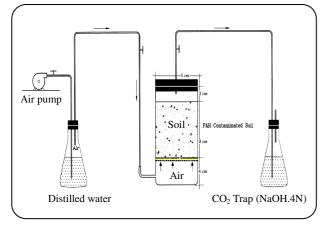
Fig. 1: Schematic diagram of pilot plant for phenanthrene contaminated soil bioremediation.
