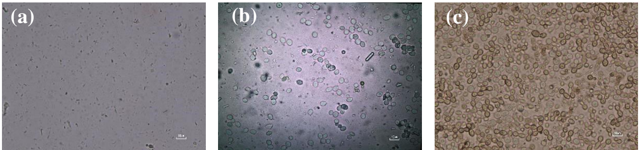
Fig 4: Microscopic images (40X magnification), (a) diluted molasses, (b) molasses after adding yeast, (c) molasses after the fermentation process
