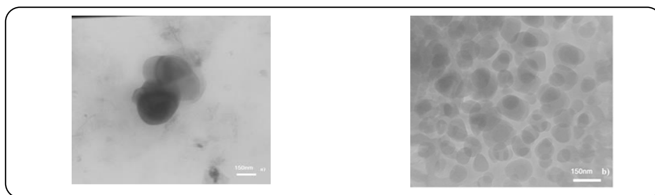
Fig.2 TEM image of permanent red 24 nano particle after separation from CTAB a) formulation contain 3% pigment b) formulation contain 2% pigment
